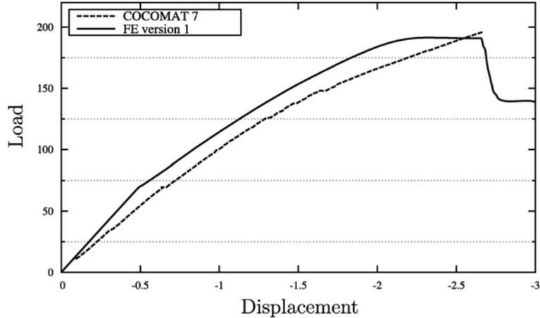
Figure 12: Load-displacement curves of the pre-damaged configuration version 1: Experiment and FE analysis
