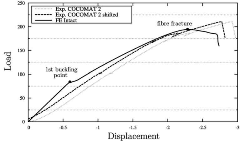
Figure 11: Load-displacement curves of the intact configuration: Experiment and FE analysis
