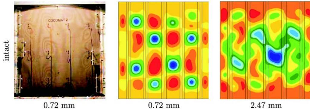
Figure 6: Out-of-plane displacements at applied shortening. Left: Intact panel. Middle and Right: FE-Results.
