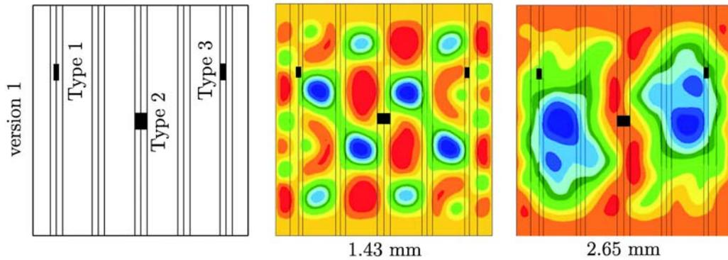
Figure 10: Pre-damaged configuration V1: Initial damage configuration and contour plots including the current state of debonding
