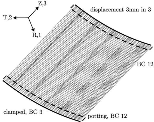
Figure 5: Generated four-node, thick shell element mesh and boundary condition (BC)
