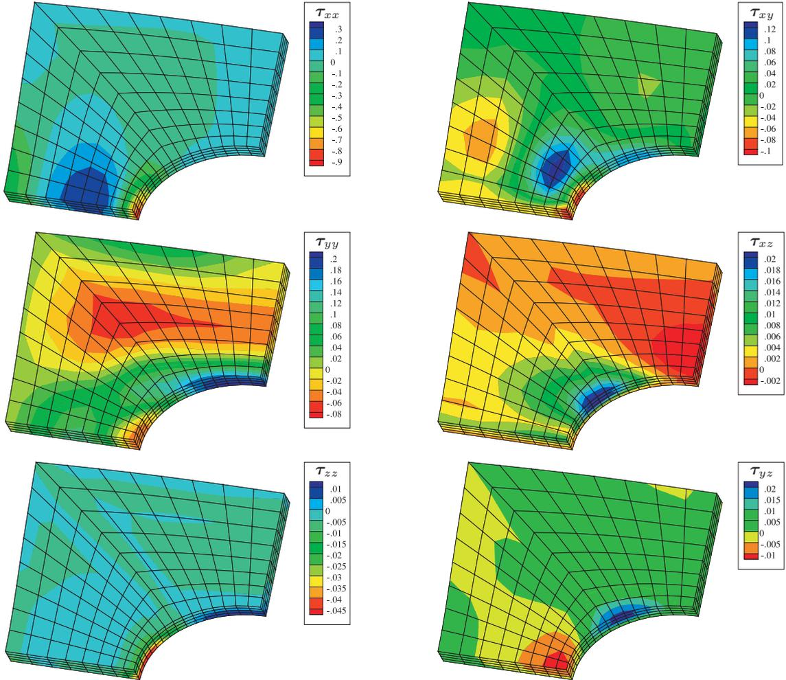
**Figure 10:** In each case  $\eta_{iso} = 1 \text{ N s mm}^{-2}$  in the deformed configuration: counterclockwise from top left:  $\tau_{xx}$ ,  $\tau_{yy}$ ,  $\tau_{zz}$ ,  $\tau_{yz}$ ,  $\tau_{xz}$ , and  $\tau_{xy}$  in  $[\text{N}/\text{mm}^2]$ .
