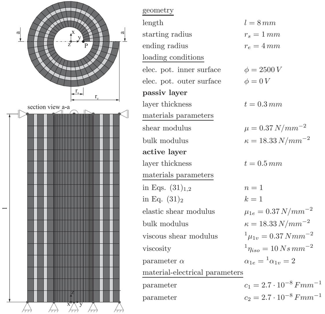
**Figure 12:** Geometry, finite element mesh, loading conditions and material parameters of the actuator
