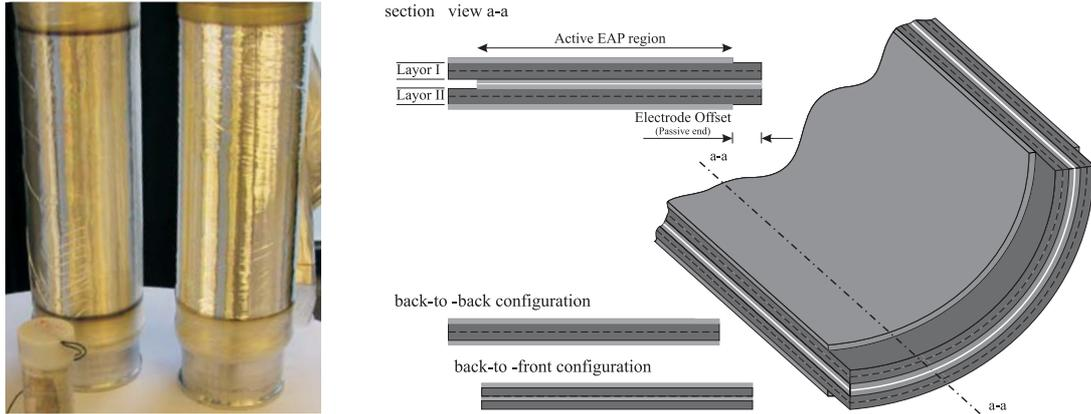
**Figure 11:** Unclad InLastor<sup>®</sup> from Danfoss Polypower A/S, Denmark (left) and schematic structure of a four-layer composite EAP laminate (right).
