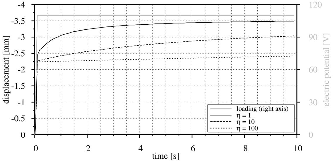
**Figure 8:** Retardation curves for the different retardation times  ${}^1\eta_{iso} = 1 \text{ N s mm}^{-2}$ ,  ${}^1\eta_{iso} = 10 \text{ N s mm}^{-2}$  and  ${}^1\eta_{iso} = 100 \text{ N s mm}^{-2}$ .
