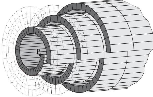
**Figure 13:** The nonlinear visco-electroelastic elements have dark shading and the electric loaded surface (active layer) has light shading. The nonconducting elements (passive layer) between the active layers are not drawn
