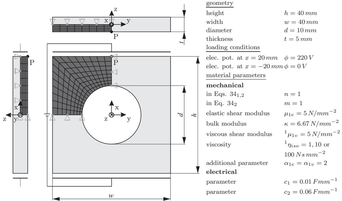
**Figure 6:** Geometry, finite element mesh (left); loading conditions and material parameters (right) of the plate
