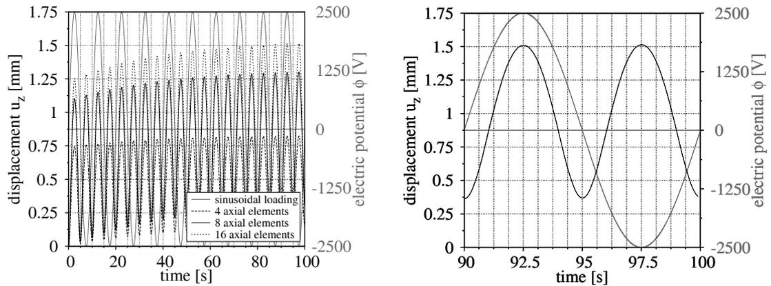
**Figure 14:** Right: displacement  $u_z$  for variable number of axial elements by frequency of  $f_1 = 0.1 Hz$ . Left: displacement  $u_z$  for the first 10 s loaded by 2500 V. For both graphs  $f_1 = 0.1 Hz$  and 16 axial elements are used
