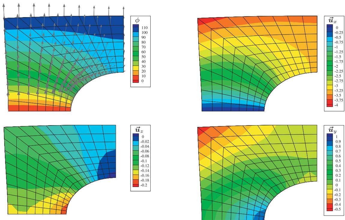
**Figure 9:** Electric potential  $\phi$  in [V], the electric displacement  $\vec{d}$  (vectors) (top left) and the displacements in x, y, z-direction in [mm] in the deformed configuration for  $\eta_{iso} = 1 \text{ N s mm}^{-2}$
