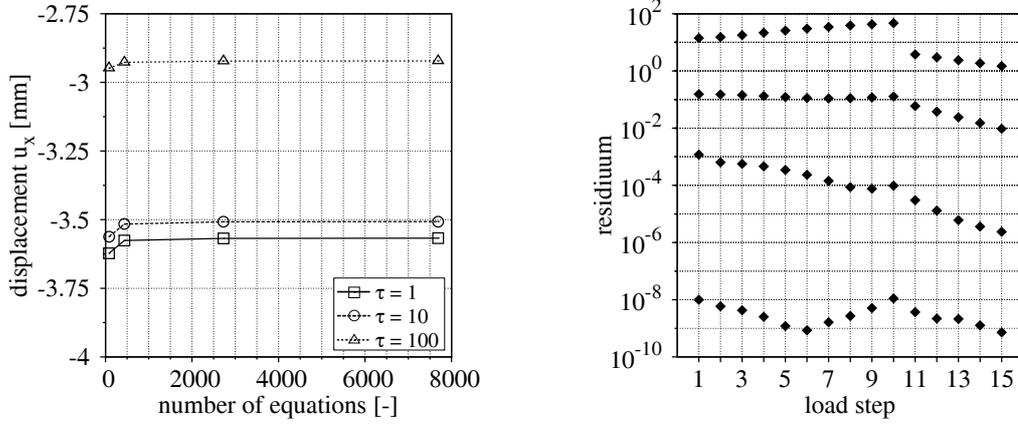
**Figure 7:** Convergence of displacement measured at point P of the plate with increasing number of elements for  ${}^1\eta_{iso} = 1 \text{ N s mm}^{-2}$ ,  ${}^1\eta_{iso} = 10 \text{ N s mm}^{-2}$  and  ${}^1\eta_{iso} = 100 \text{ N s mm}^{-2}$  (left); Residuum order exemplary for the first 15 load increments and  ${}^1\eta_{iso} = 1 \text{ N s mm}^{-2}$  (right).
