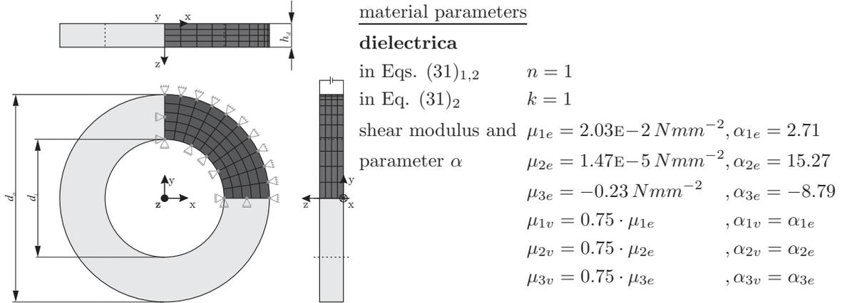
**Figure 17:** Finite element mesh and material parameters of the actuator. Not drawn to scale.
