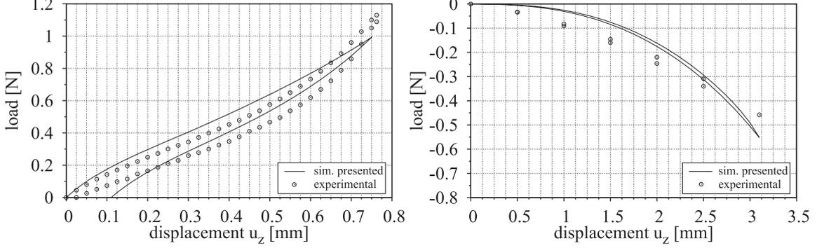
**Figure 18:** Uniaxial pull test of the dielectric elastomer (left) and of the considered actuator without electrodes (right) to indicate the material parameters. Experimental results are taken from [35] and [33], respectively.
