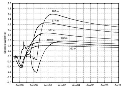
Fig. 3: Long term stress evolution for different elevations.
