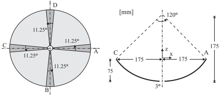
Figure 14: Geometry of the parabolic antenna.
