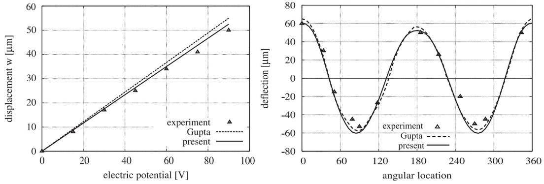
Figure 12: Electric potential - displacement curve of the antenna for the actuator usage under symmetrical loading (a) and deflection for actuator usage under asymmetric loading [150V/75V](b).
