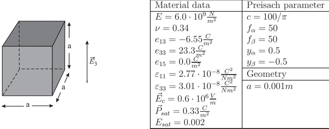
Figure 16: Geometry, material and Preisach parameter for the test specimen.
