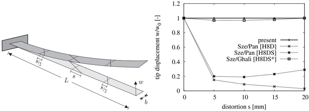
Figure 8: System and results for the bimorph with distorted mesh.
