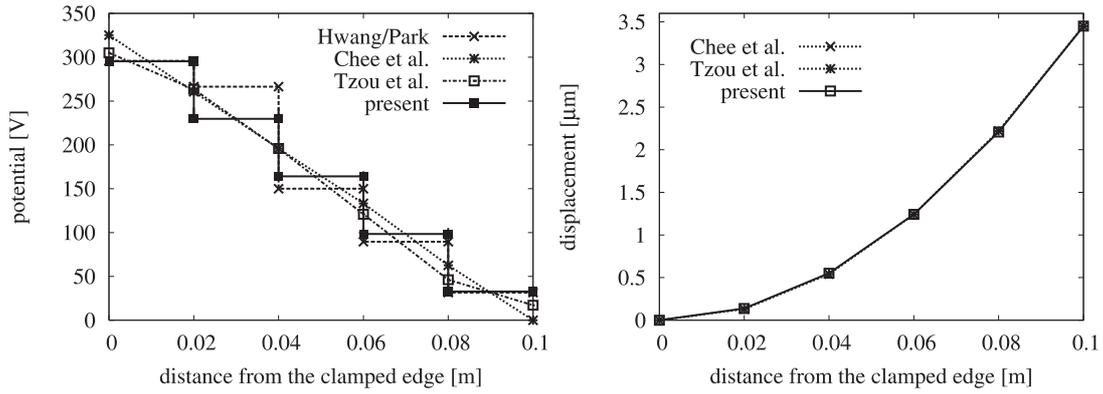
Figure 7: Distribution of the electric potential along the bimorph structure for sensor usage (a) and deflection of the bimorph due to actuator loading (b).
