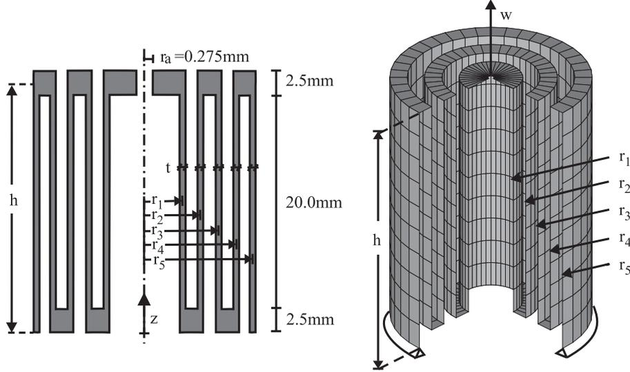
Figure 21: Geometry and finite element discretization of the telescopic cylinder.
