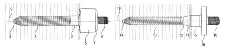
Innovative and advantageous design detail is the option to lengthen the overgrowth section by screw on of further adapter section to extend the service life of the connection. The limb or at least ist part in cotact with wood are out of stainless steel of maximum quality to prevent biochemical interactions and corrosion. An accurate pilot hole and tree resing filling are essential for the installation. The penetration ratio ought to stay as little as possible.
