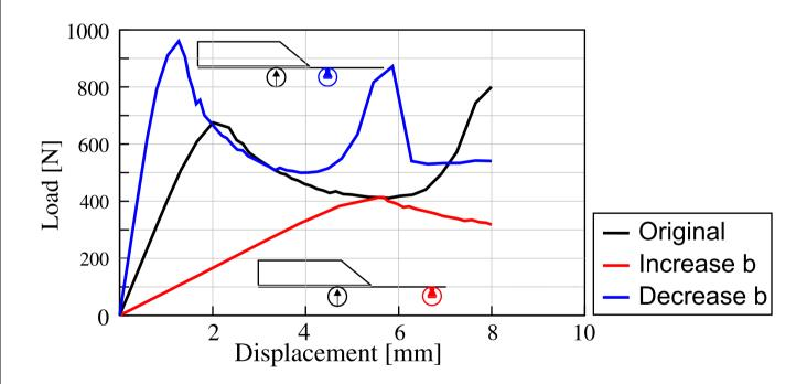
Normal loarding was highly influenced by the roller position, sliding delamination was affected by the laminate thickness. Both simulations reacted similar to changes in CZMs and a noticeable feature is that as soon the load drops, the delamination area increases massively.
