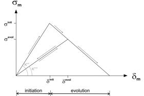
This bi-linear failure mechanism shows two distinct parts: *initiation* and *evolution*. A scalar damage indicator D maps the degradation and appears in the actual stress tensor t in order to relate to the initial stress tensor  $\overline{t}$ .
